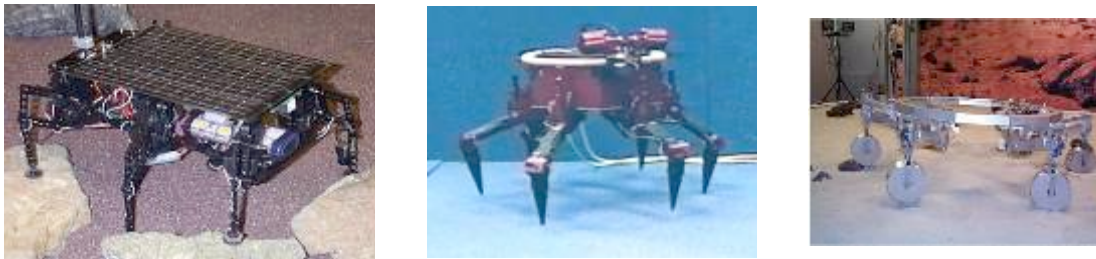
Figure 14-1 Several Generations of NASA/JPL “Hexabot” from the mid-1990s
